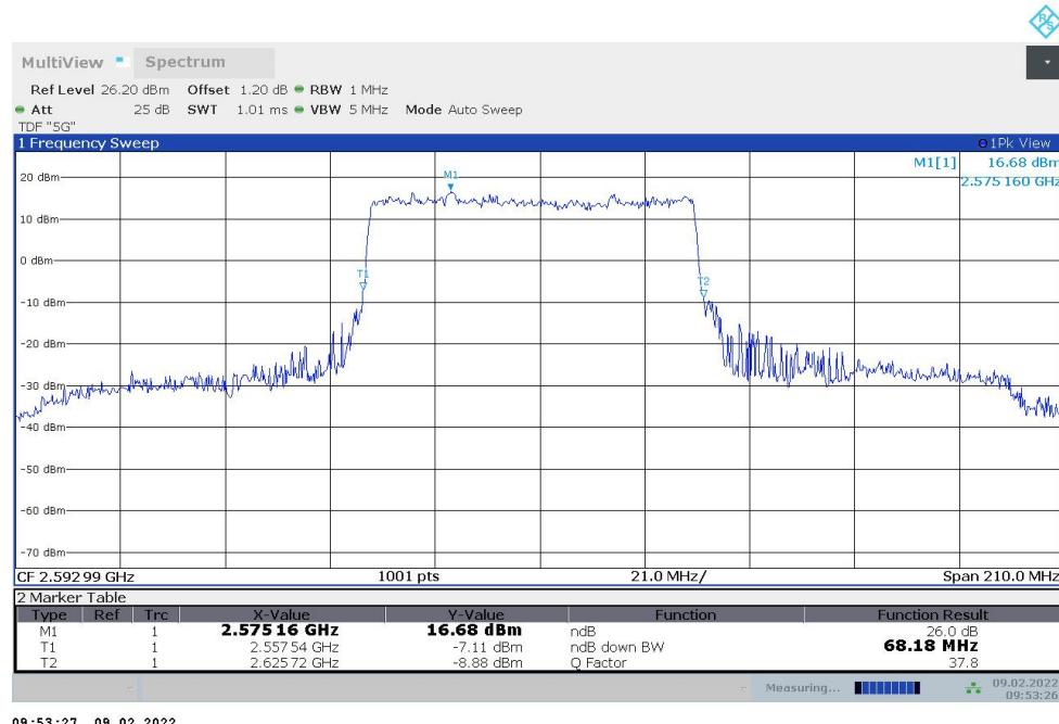
**n41,70MHz Bandwidth,DFT-s-QPSK (-26dBc BW)**
