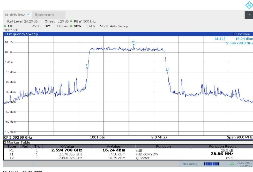
**n41,30MHz Bandwidth,DFT-s-QPSK (-26dBc BW)**
