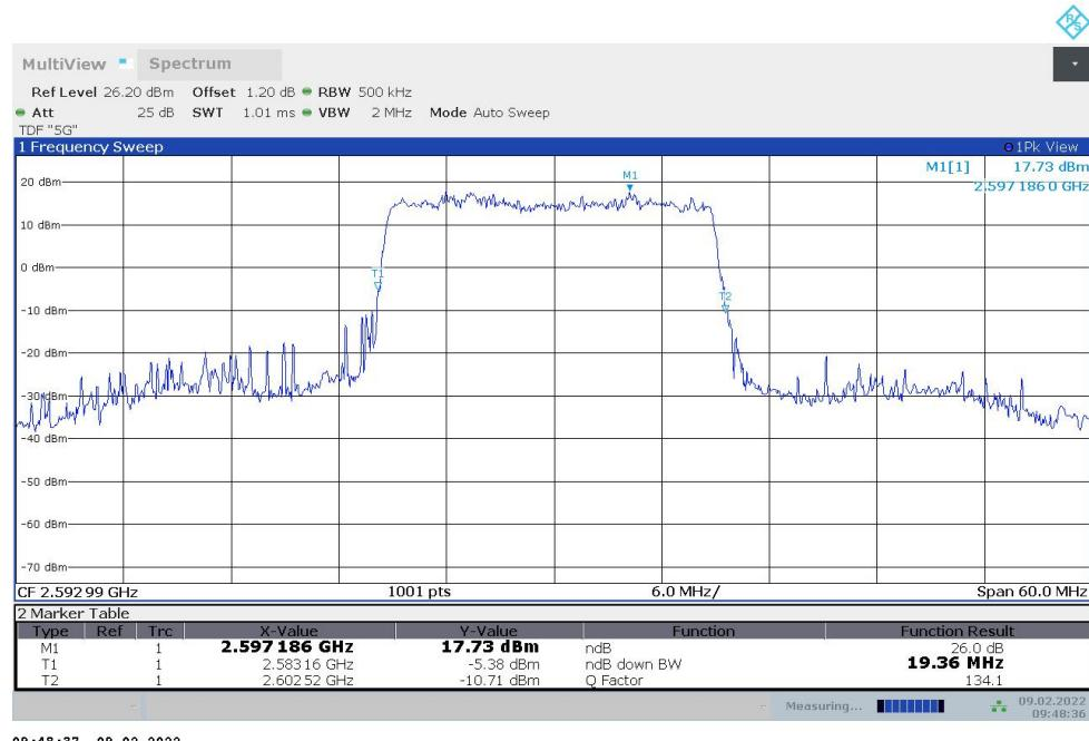
**n41,20MHz Bandwidth,DFT-s-QPSK (-26dBc BW)**
