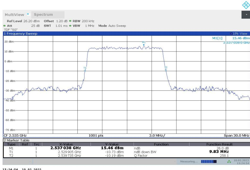
**n7,10MHz Bandwidth,DFT-s-QPSK (-26dBc BW)**
