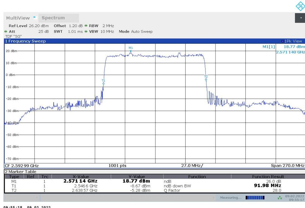
**n41,90MHz Bandwidth,DFT-s-QPSK (-26dBc BW)**
