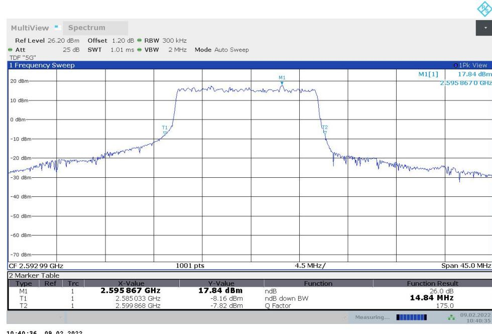
**n41,15MHz Bandwidth,DFT-s-QPSK (-26dBc BW)**
