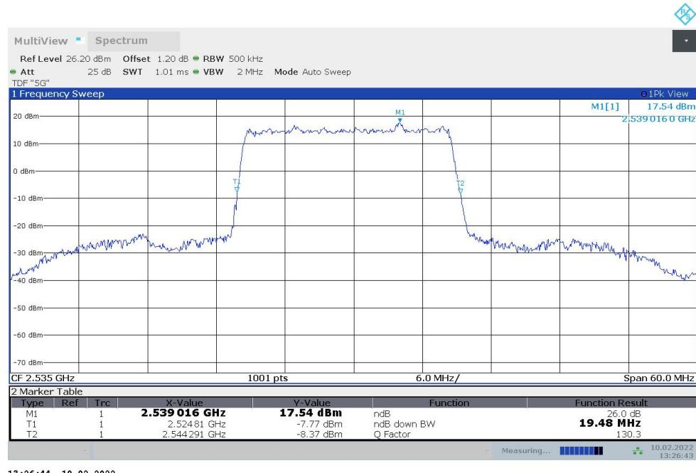
**n7,20MHz Bandwidth,DFT-s-QPSK (-26dBc BW)**
