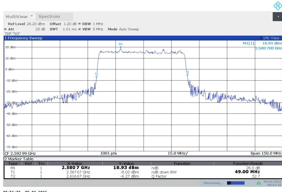
**n41,50MHz Bandwidth,DFT-s-QPSK (-26dBc BW)**
