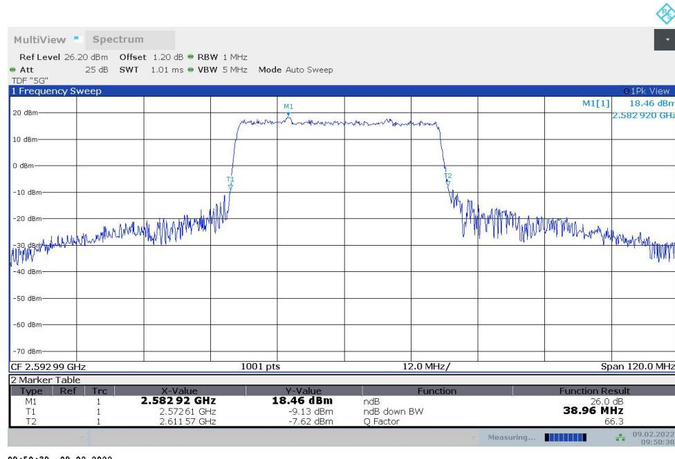
**n41,40MHz Bandwidth,DFT-s-QPSK (-26dBc BW)**
