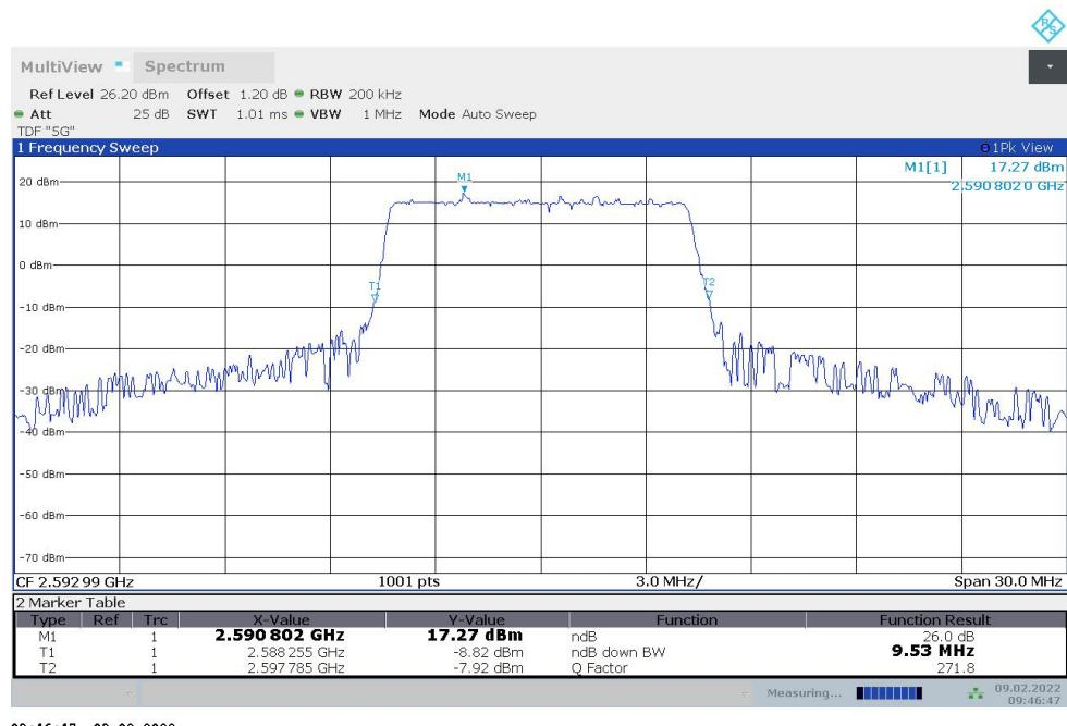
**n41,10MHz Bandwidth,DFT-s-QPSK (-26dBc BW)**
