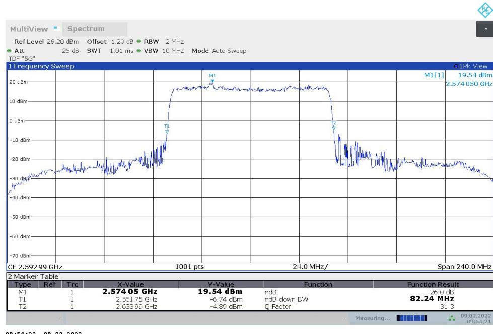
**n41,80MHz Bandwidth,DFT-s-QPSK (-26dBc BW)**
