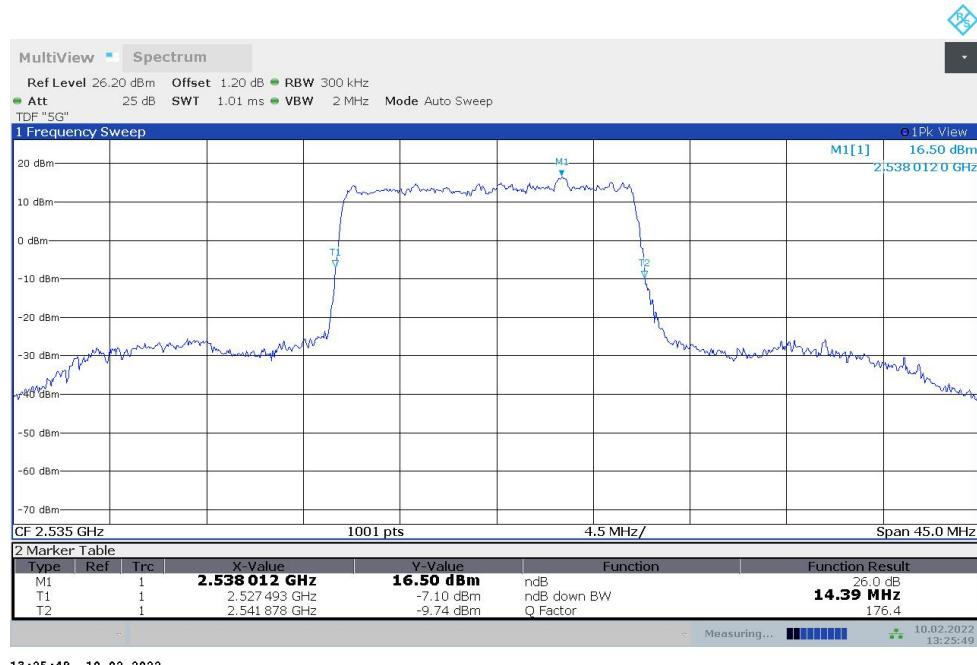
**n7,15MHz Bandwidth,DFT-s-QPSK (-26dBc BW)**
