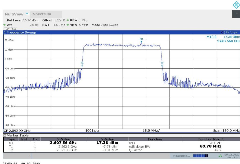
**n41,60MHz Bandwidth,DFT-s-QPSK (-26dBc BW)**
