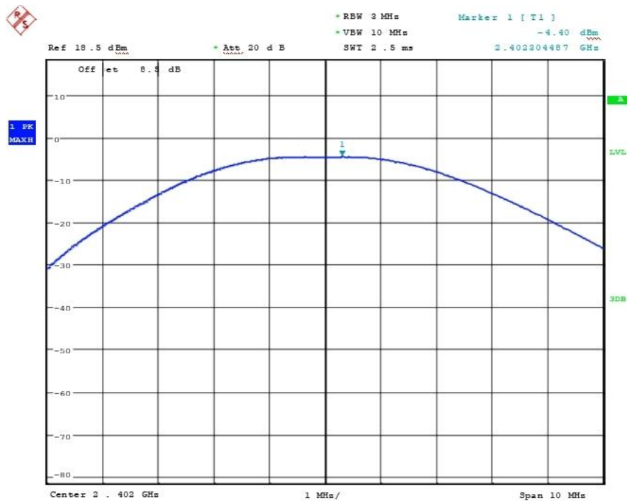
Fig.4. Peak Conducted Output Power: BLE, 2Mbps, Channel 0,
