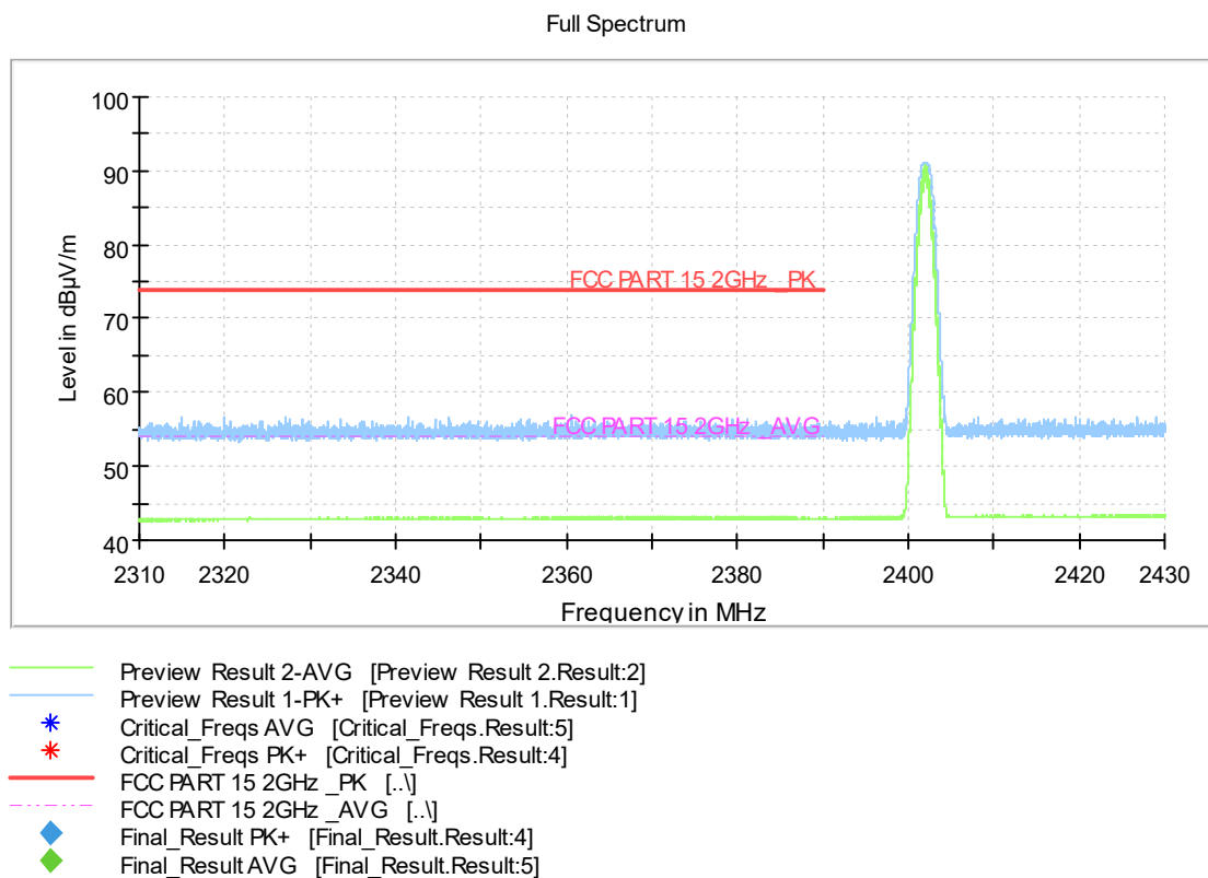
Fig.9. Frequency Band Edges: BLE 4.0, GFSK, 2402 MHz, Hopping Off, 2.38 GHz – 2.45GHz
