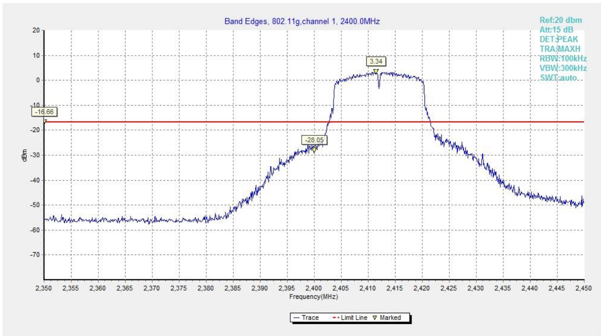
Fig.A.5.1.3 Band Edges (802.11g, Ch 1)
