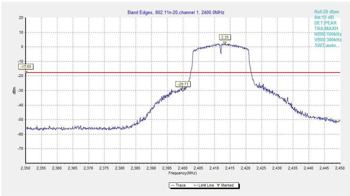
Fig.A.5.1.5 Band Edges (802.11n-HT20, Ch 1)
