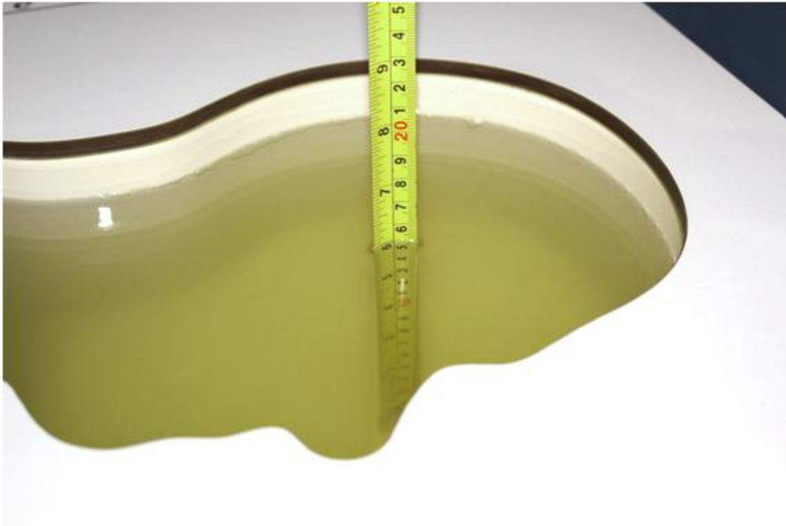
Picture 7-7 Liquid depth in the Head Phantom (3500-3900 MHz)
