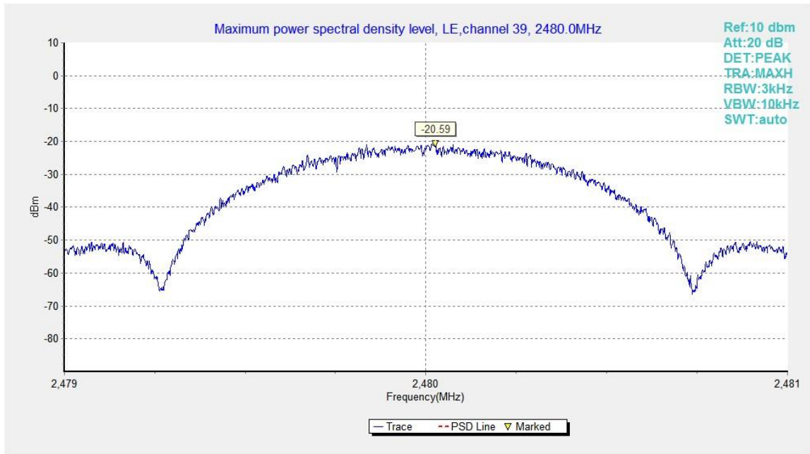
Fig.33. Maximum Power Spectral Density Level Function: GFSK, 2480 MHz
