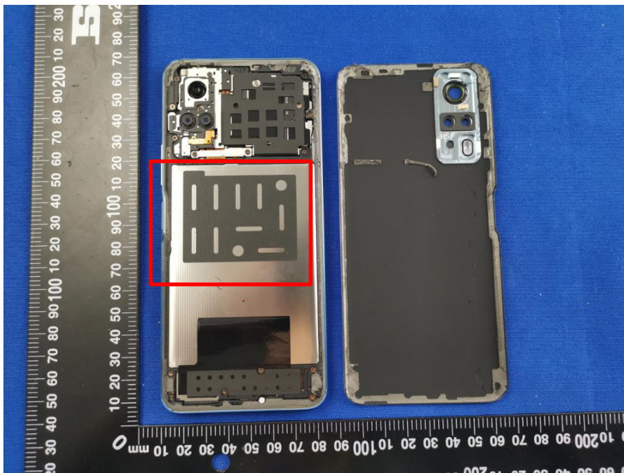
EUT UNCOVER VIEW_BATTERY COVER WITH FOAM GASKET
