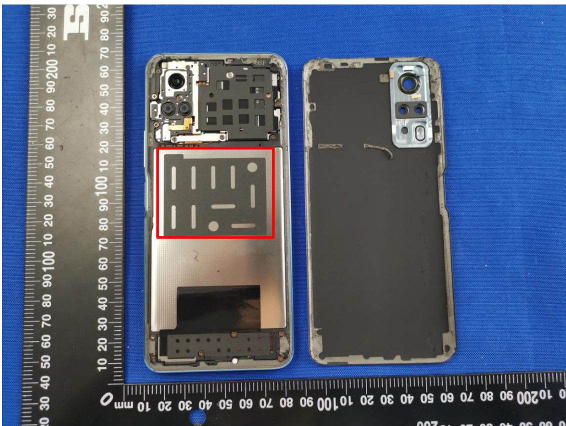
EUT UNCOVER VIEW_BATTERY COVER WITH FOAM GASKET
