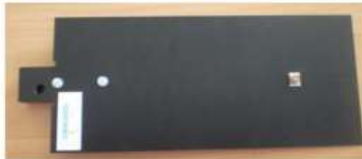
Figure 1 – MVG COMOHAC Validation Dipole
