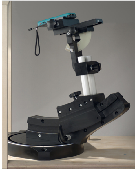
F-2. Device Holder for Transmitters
