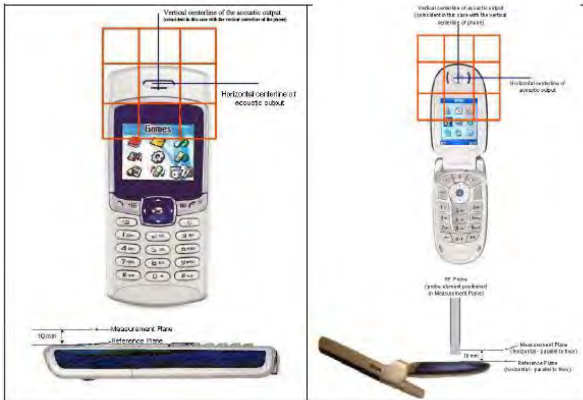
Reference and plane for RF emission measurements
