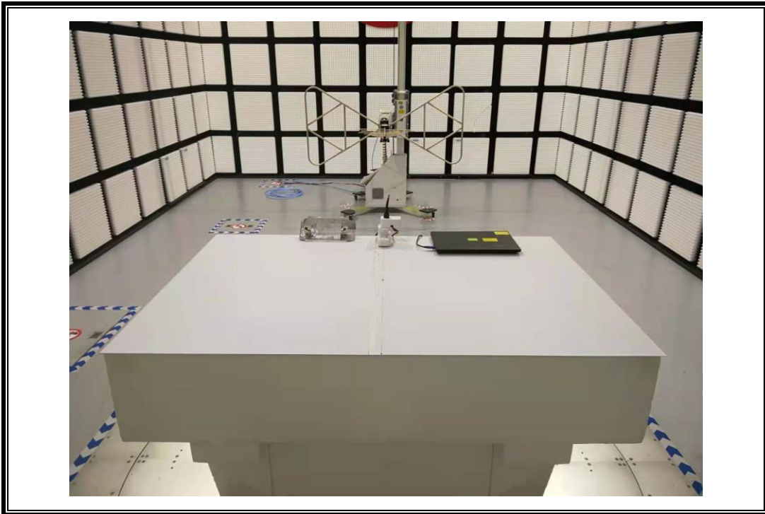
RADIATED RF MEASUREMENT SETUP (30MHz ~ 1 GHz)
