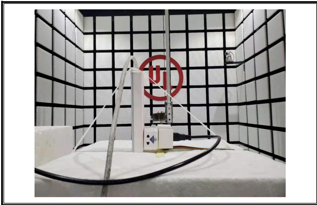
POWERLINE CONDUCTED EMISSIONS MEASUREMENT SETUP
