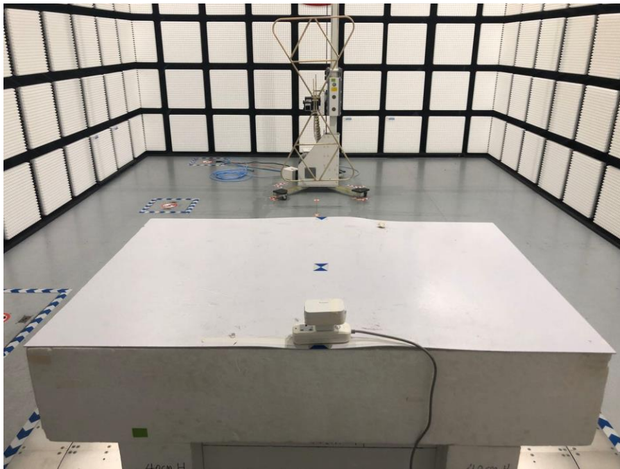
RADIATED RF MEASUREMENT SETUP (30MHz~1GHz)
