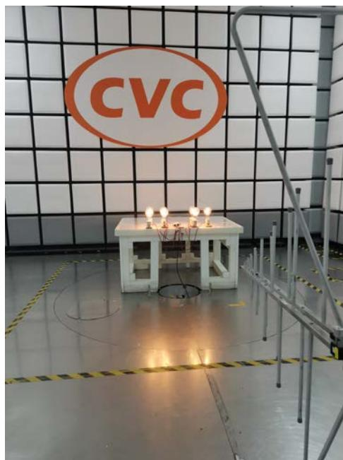
(2) Radiated spurious emission Test Setup(Above 1GHz)
