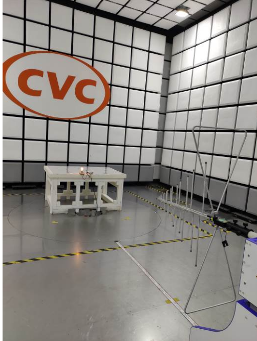
(2) Radiated spurious emission Test Setup(Above 1GHz)
