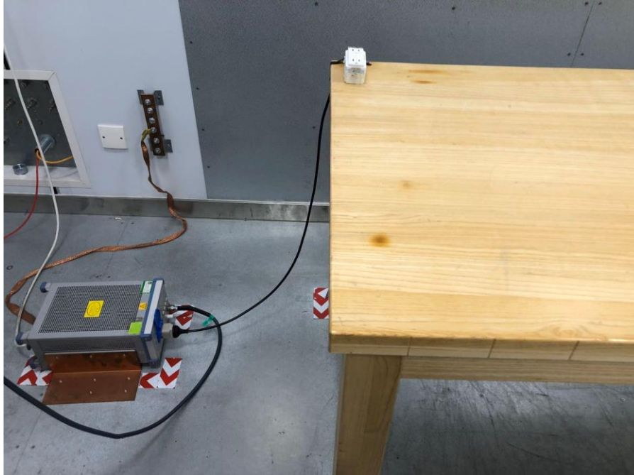
POWERLINE CONDUCTED EMISSIONS MEASUREMENT SETUP
