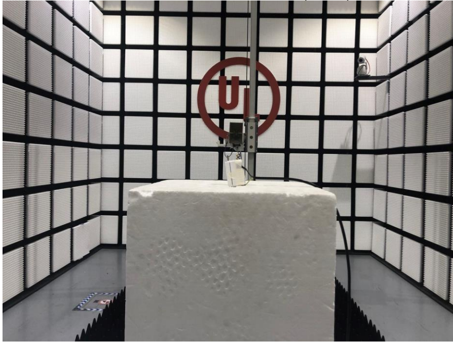
RADIATED RF MEASUREMENT SETUP (30MHz~1GHz)
