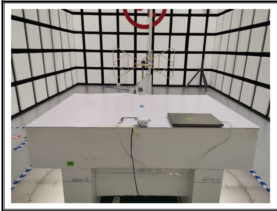
RADIATED RF MEASUREMENT SETUP (Below 30MHz)
