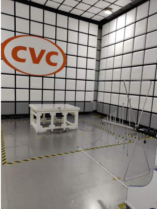
(1) Radiated spurious emission Test Setup(Below 1GHz)
