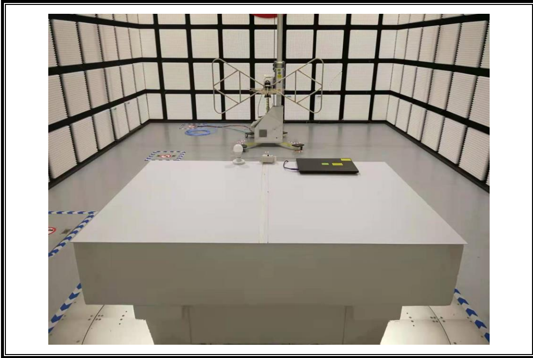
RADIATED RF MEASUREMENT SETUP (30MHz ~ 1 GHz)
