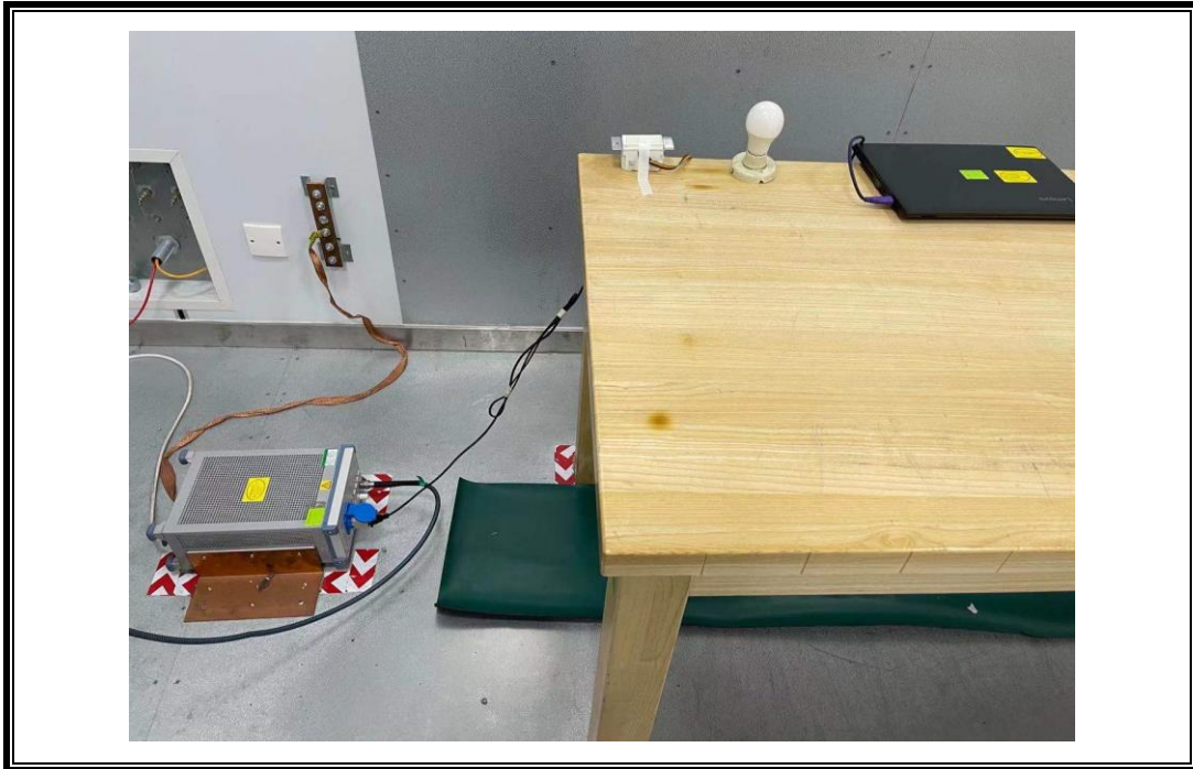
POWERLINE CONDUCTED EMISSIONS MEASUREMENT SETUP
