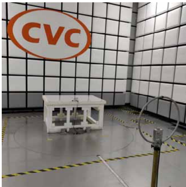
(1) Radiated spurious emission Test Setup-1(9KHz~30MHz)
