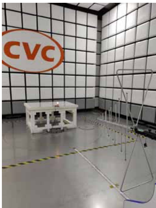
(2) Radiated spurious emission Test Setup-2(Below 1GHz)
