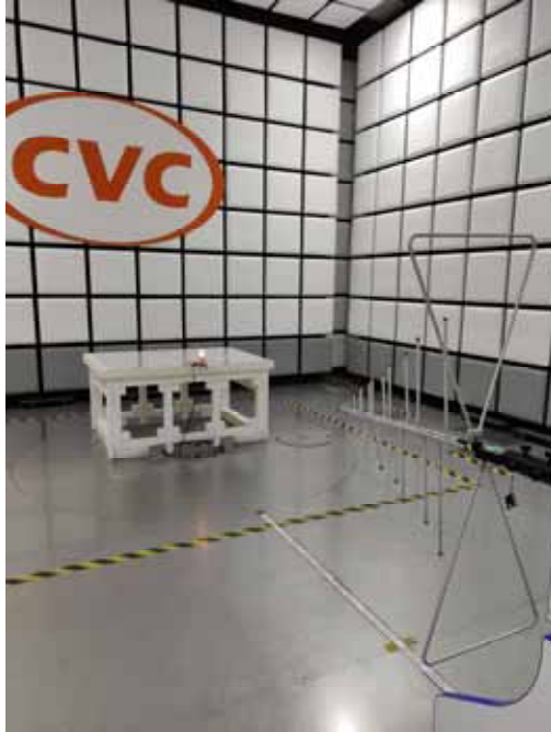
(2) Radiated spurious emission Test Setup(Above 1GHz)
