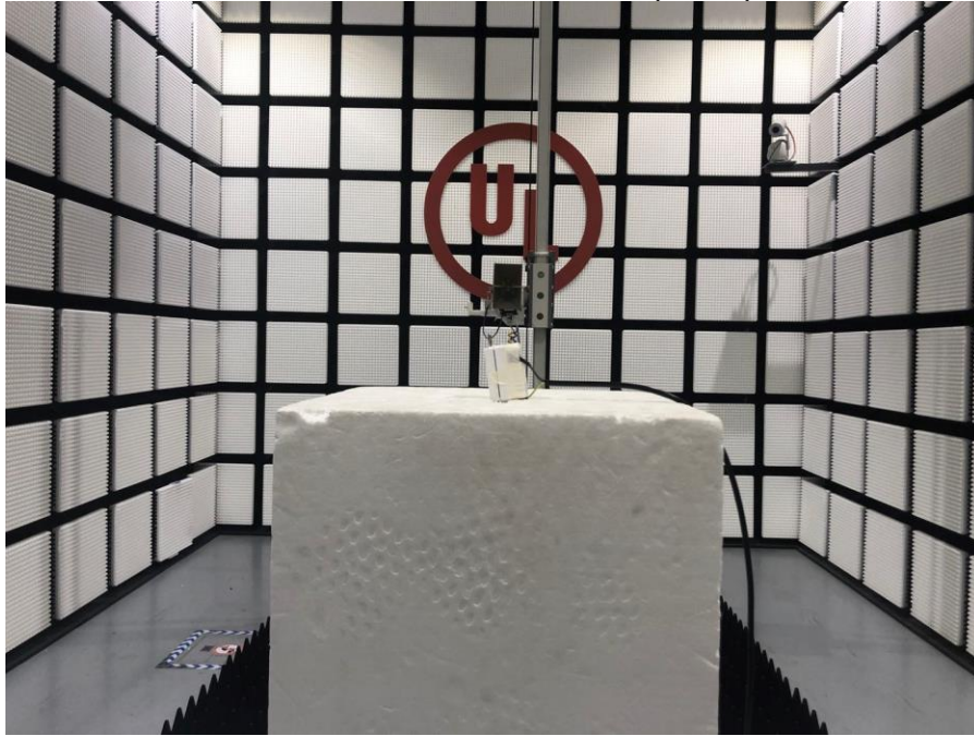
RADIATED RF MEASUREMENT SETUP (30MHz~1GHz)
