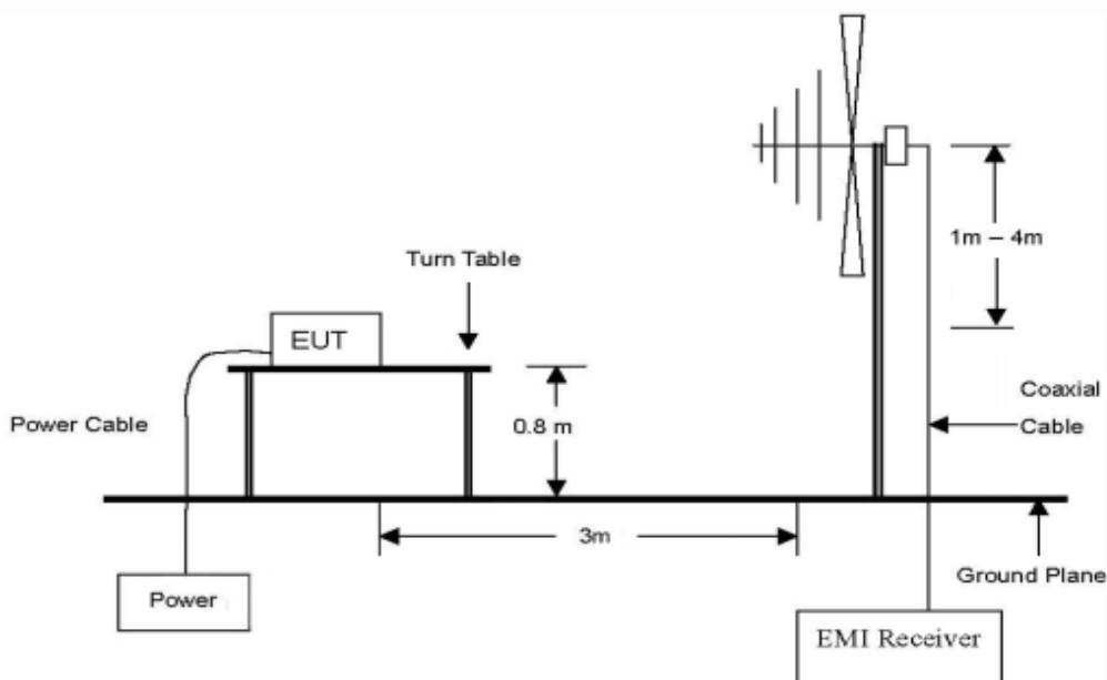
The diagram below shows the test setup that is utilized to make the measurements for emission. The
