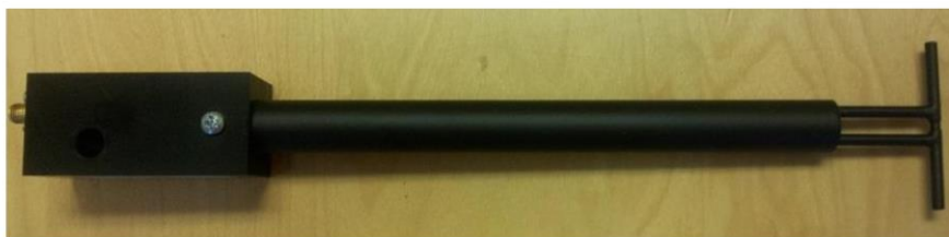
Figure 1 – MVG COMOSAR Validation Dipole
