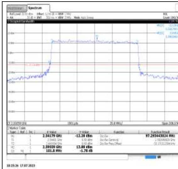
1-N41-PC3-30-100-M-6-CP-16QAM- Outer_Full-273@0-Ant1-97.293-101.800- ≤100-PASS
