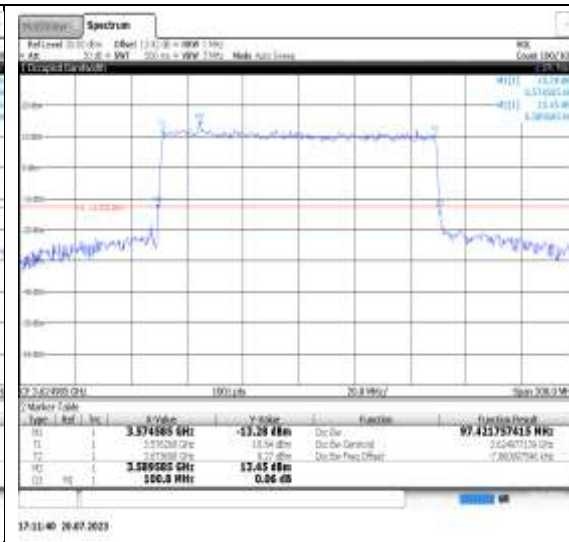
1-N48-PC3-30-100-M-7-CP-64QAM- Outer_Full-273@0-Ant1-97.422-100.800- ≤100-PASS
