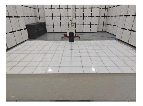
Set-up for Radiated Spurious Emission, Below 1GHz
