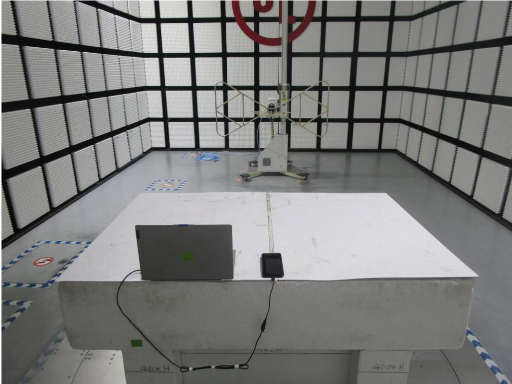
Set-up for Radiated Spurious Emission, Above 1GHz
