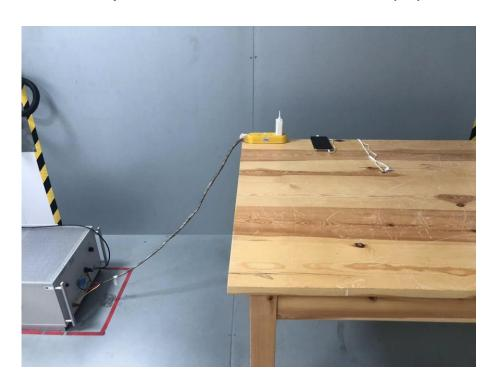
Set-up for Radiated Emission (RE), Below 1GHz
