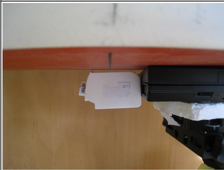
5 mm separation distance to phantom - Vertical Back
