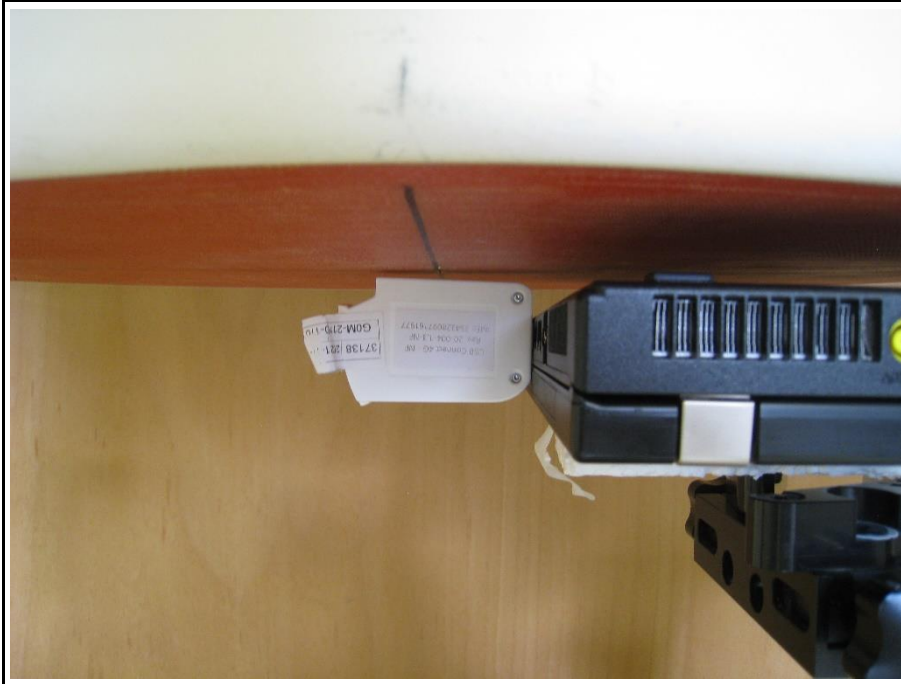
5 mm separation distance to phantom - Vertical Front
