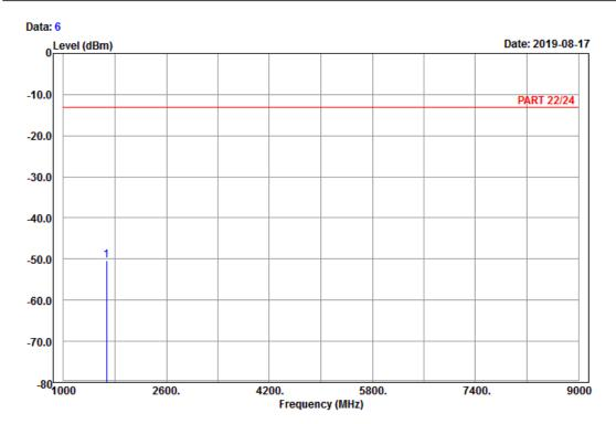
Site : 966 chamber 1 Condition: PART 22/24 Vertical Remark : Band V\_Link\_M-Ch
