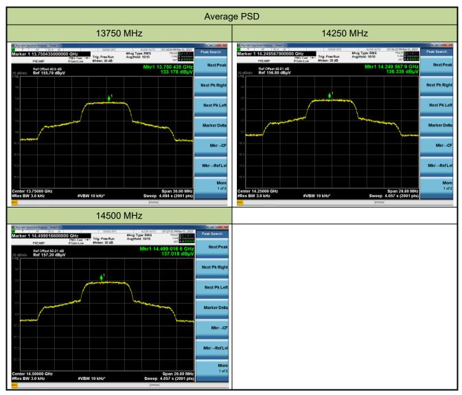
Note 1: The measured level was in  $dB\mu V/m$ , which had compensated cable loss (dB), antenna factor (dB/m) in SA's Ref offset, but showed  $dB\mu V$  in SA's screen.
