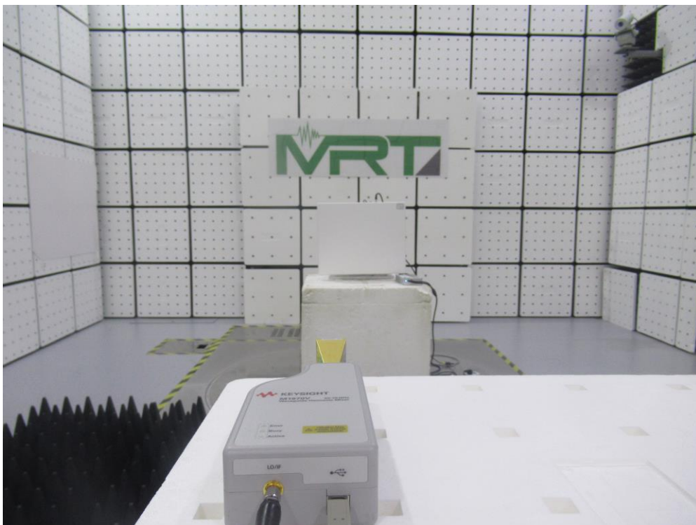
Description: Radiated Spurious Emission Test Setup of 50GHz ~ 75GHz
