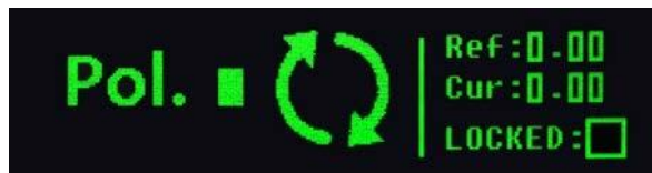
Figure 5-2-1-3: Polarization adjustment display
