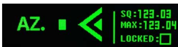
Figure 5-2-1-5: Azimuth adjustment display
