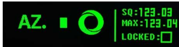
Figure 5-2-1-6: Azimuth adjustment is completed
