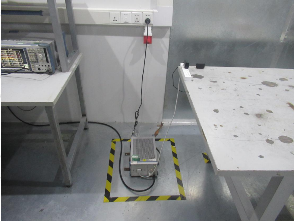
Photo of Conducted Emission Measurement
