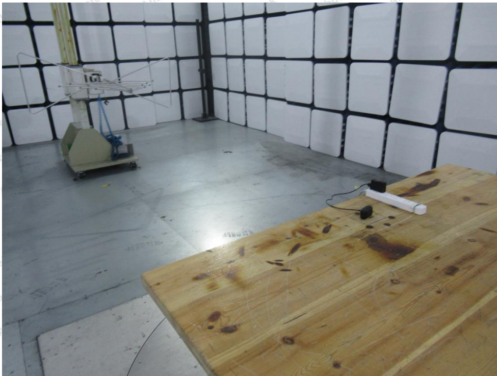
Photo of Radiation Emission Test
