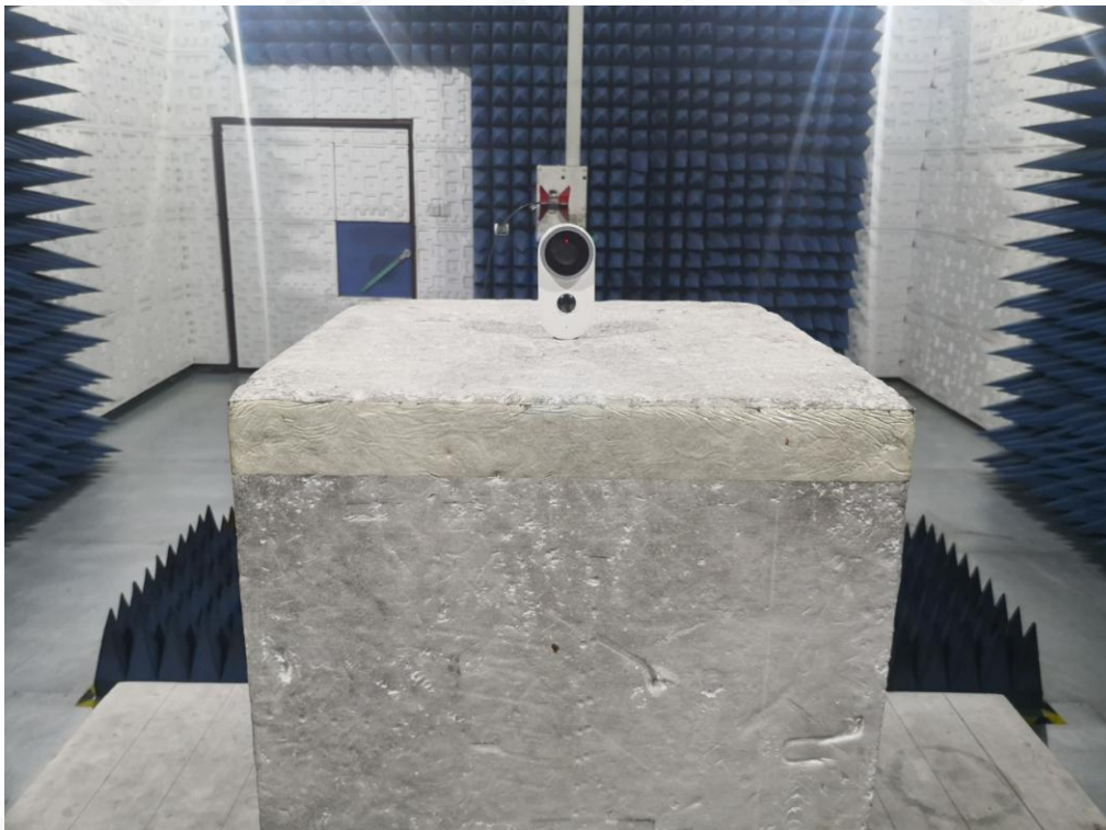
FCC RADIATED EMISSION TEST SETUP ABOVE 1GHZ
