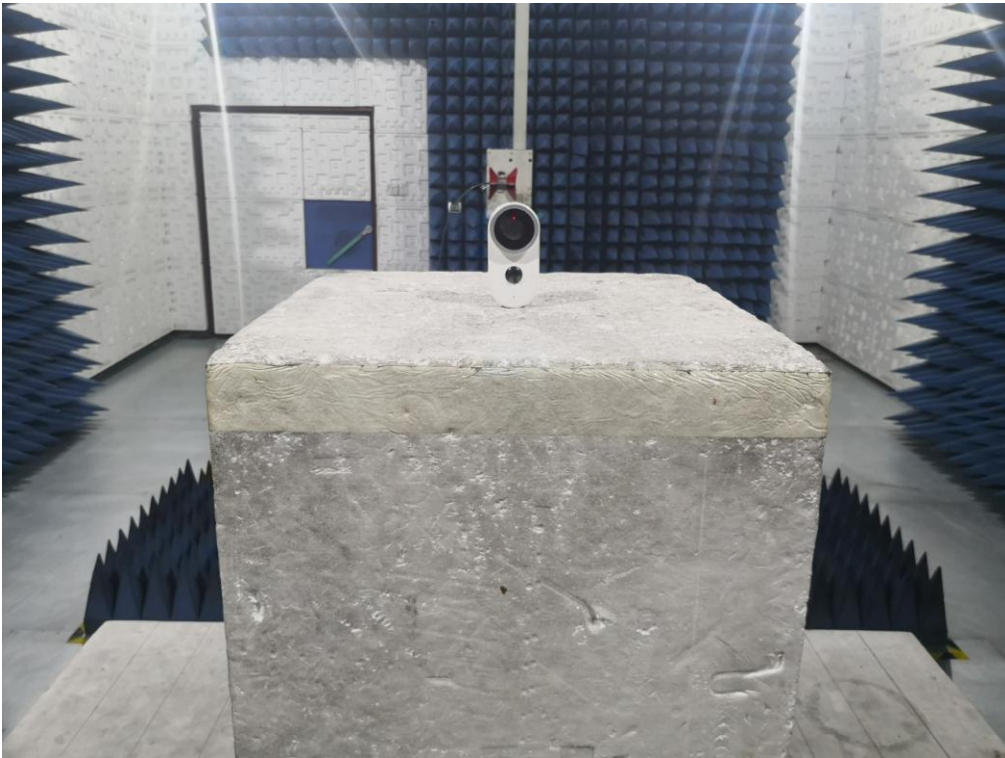
FCC RADIATED EMISSION TEST SETUP ABOVE 1GHZ
