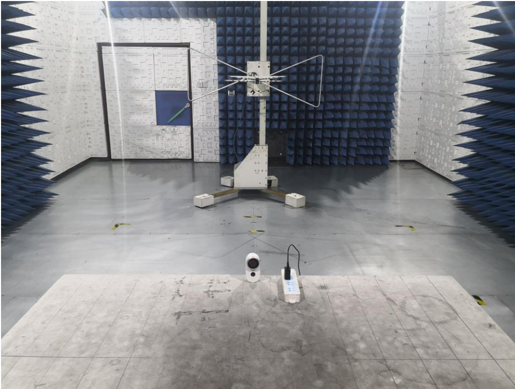
FCC RADIATED EMISSION TEST SETUP ABOVE 1GHZ
