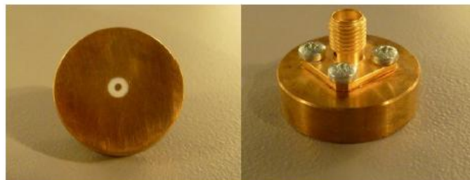
Figure 1 – MVG LIMESAR Dielectric Probe
