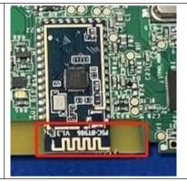
The antenna is PCB antenna. The best case gain of the antenna is 2 dBi.
