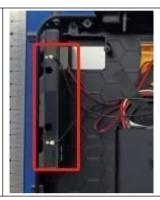
The antenna is FPC antenna.5.1G:3.73dBi,5.8G:4.55dBi
