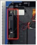
The antenna is FPC antenna. Ant 1: 3.72dBi
