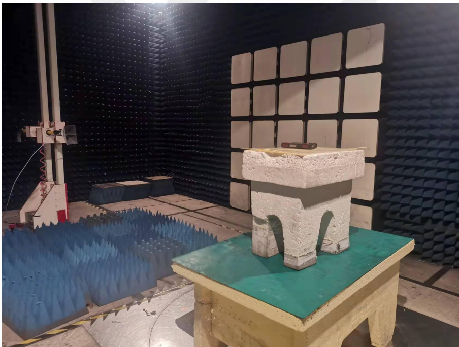
Spurious Emission Test Setup (Above 1GHz)
