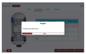
c) Learning: with this function, the sensor ID can be written into the vehicle ECU for sensor identification.
