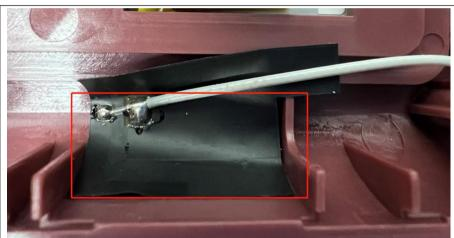
The antenna is FPC antenna. The best case gain of the antenna is 3.34 dBi.
