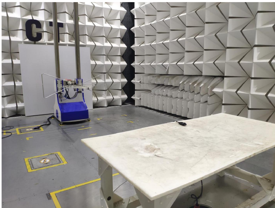
Radiated spurious emission Test Setup-2(Below 1GHz)
