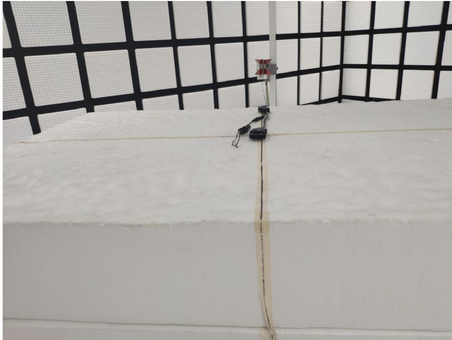
Radiated spurious emission Test Setup-3(Above 1GHz)
