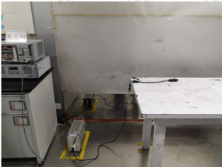
Conducted Emissions Test Setup
