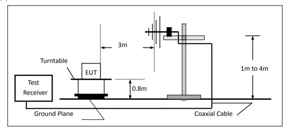
(c) For radiated emissions above 1000MHz
