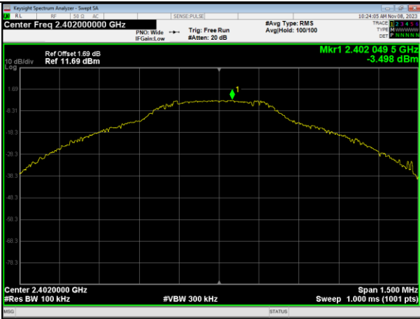
GFSK on Channel 39
