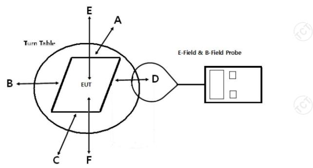
Note: Measurements should be made from all sides of the primary/client pair, with the 0 cm or 10 cm measured from the center of the probe(s) to the edge of the device.
