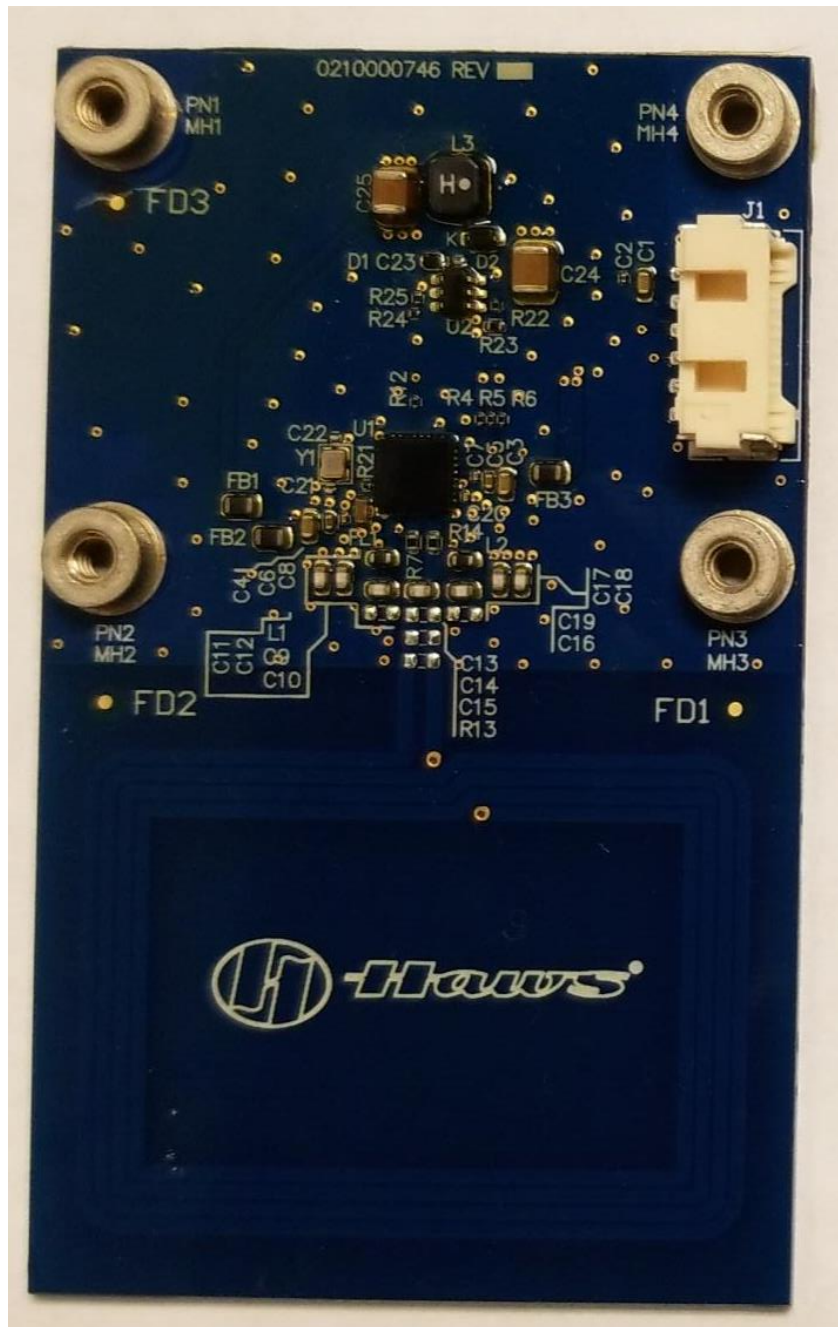
Figure 5 - RFID Board Front (0210000745)
