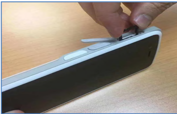
Figure 2-3 Take out the SD Tray when it pops up.
