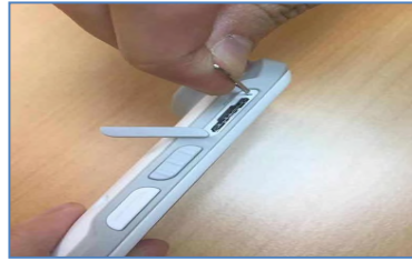
Figure 2-2 Insert the ejector tool or a metal pin into the small hole
