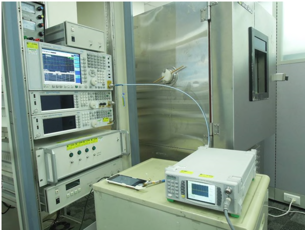
Photograph 4: Set-up for Conducted testing
