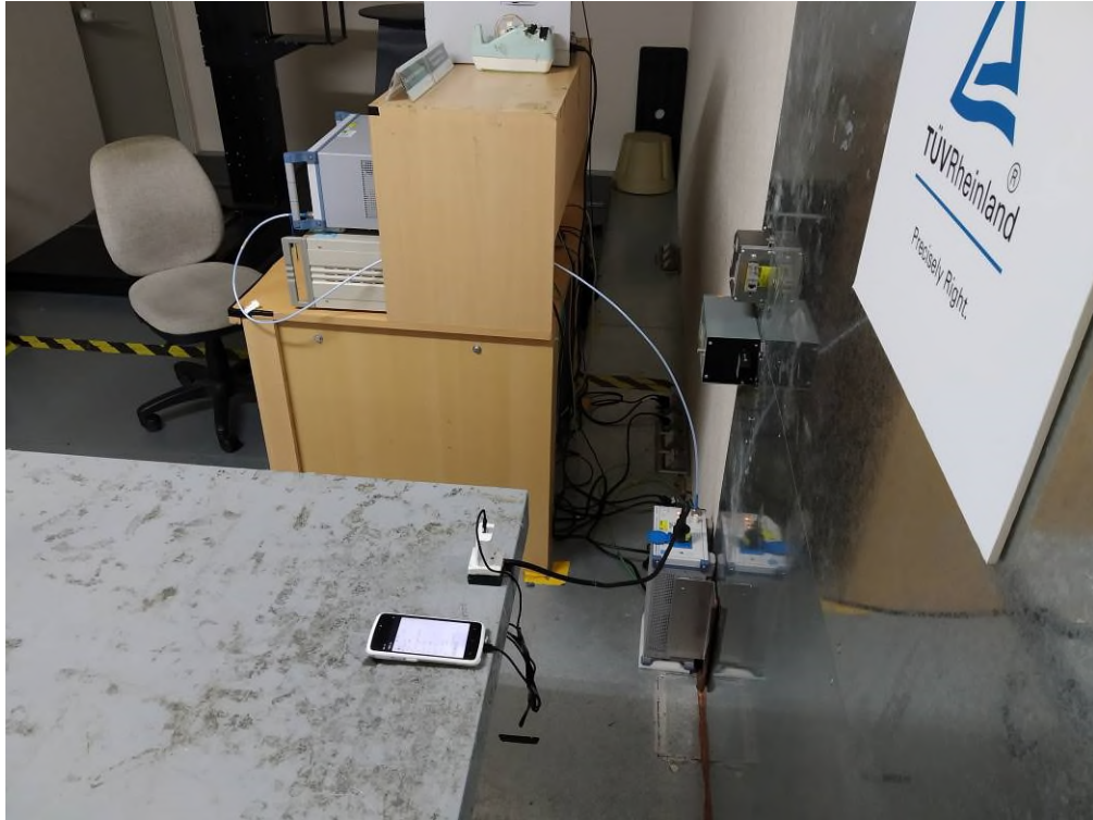
Photograph 6: Set-up for for AC Mains (Front)
