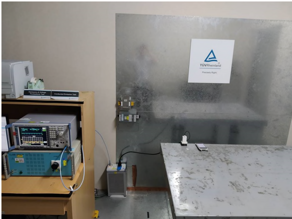
Photograph 6: Set-up for for AC Mains (Front)
